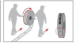
Make sure to load the coil with the arrows in the direction of deployment.
