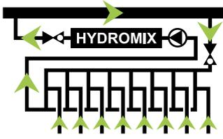
Bypass system for pressurized-line water source, with 8 dosing channels.
