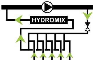
Bypass system for storage-tank water source.
