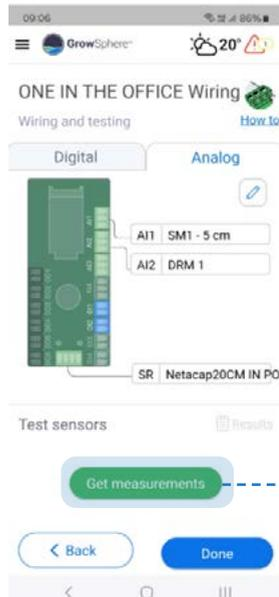
To validate correct wiring and sensor functionality, click on 'Get measurements'
